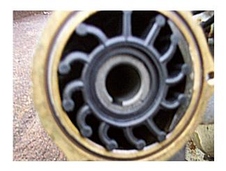
After you have the pump apart, make a note of how the impeller is laying inside of the housing. You want to make sure you put the new pump in the same orientation as the old.
