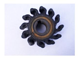
Over a long period of storage the blades will conform to the inner surface of the housing reducing efficiency of the raw water pump that can lead to problems with overheating and potentially result in engine damage. Preventative maintenance is the preferred method when it comes to things such as impellers, which are relatively inexpensive and easy to inspect and replace.
