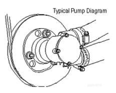
Some manufacturers recommend removing the impeller each season to prevent the rubber from becoming distorted from long term storage in the pump housing. The pump housing where the impeller spins is not a perfect circle but has somewhat of an oblong shape inside of it to create the suction as the blades spin.
